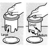
E. To fill the sink, insert the stopper so that the largest slot lines up with the switch plunger. The stopper can now be pushed down to seal the sink without starting the disposer. When the medium-sized slot in the stopper base is lined up with the switch plunger, water can drain, but tableware, etc., cannot be accidentally dropped into the disposer.
